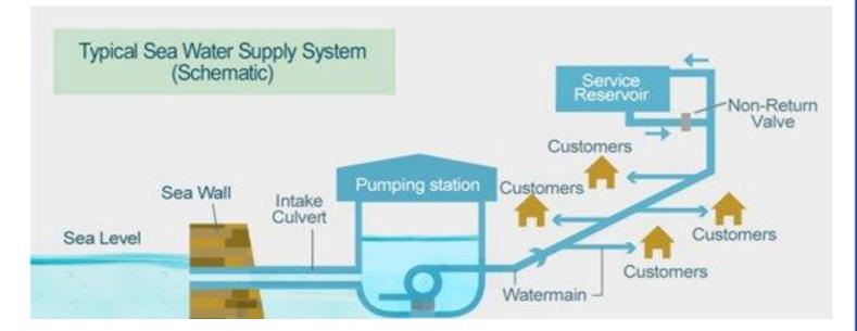
**Network**: 35 pumping stations/55 service reservoirs in the system – with a storage capacity of ~260,000 m3 and 1600km of seawater pipeline.
