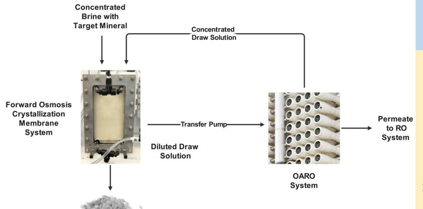
Total Energy Use for Salt Crystallization 7.5 kWh/m<sup>3</sup>
