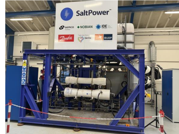
Industrial scale module test rig. 3 m 3 /hr, 80 bars 24/7
